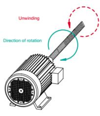
Outermost layer left-wound for operation in clockwise (right-hand) direction
