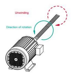
Outermost layer right-wound for operation in counter-clockwise (left-hand) direction
